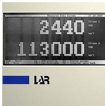
A big graphical screen; 2-stream, effluent and influent
