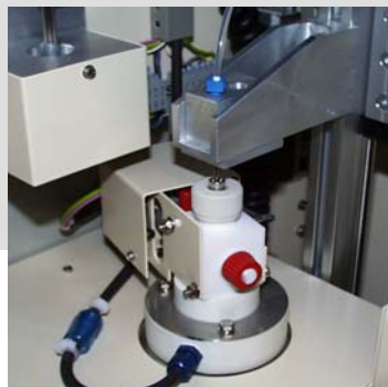
The injection port and robot with injection needle
