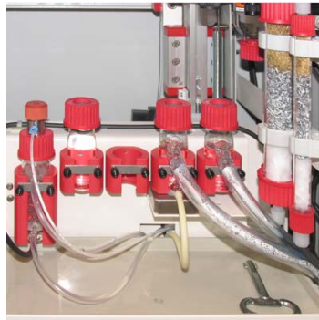
Quick-TOC-differential with TIC-reactor (left)
