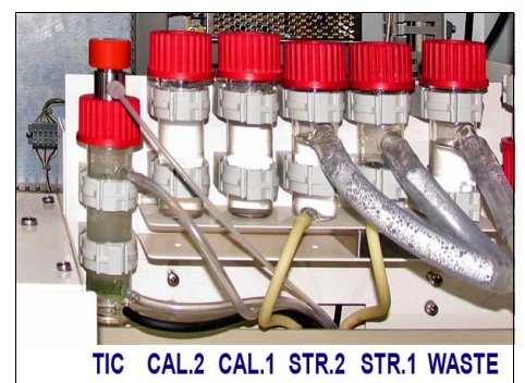
TC, TIC & TOC-analyser differential 2 streams
