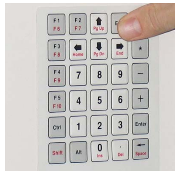
Easy menu with alphanumeric membrane keyboard
