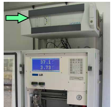
Quick-TOC & TNb analyser with chemiluminescence Nox analyser
