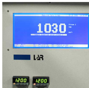
A big display shows directly the TOC or correlated COD value
