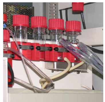
The robot will select: sample, acid solution, a standard or zero water
