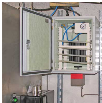
The external mounted gas permeation box
