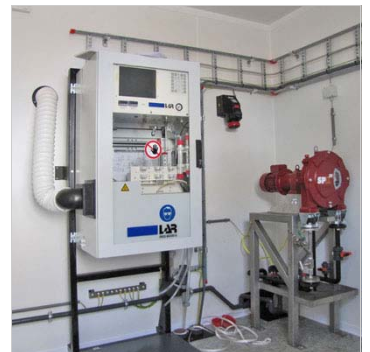
De Total Oxygen Demand analyser model Quick-COD-o
