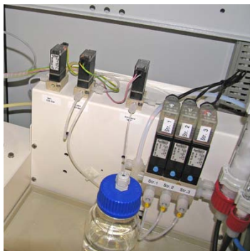
Calibration standard or Grab Sample inlet; 3-stream analyser
