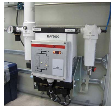
Zero air supply based on pressure swing absorption
