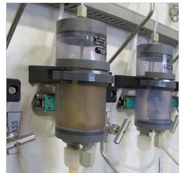
Overflow vessels with level alarm sensors detect sample supply
