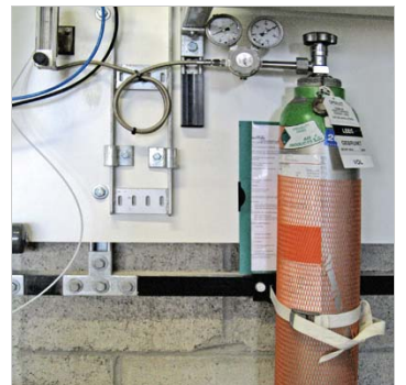
Validation via a stable certified gas mixture (CO 2 or CH 4 in N 2 )
