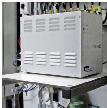
Zero Air supply with catalytical oxidation and PSA
