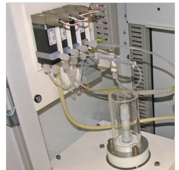
The Quick-TOC-condensate LAR with multi-loop injection
