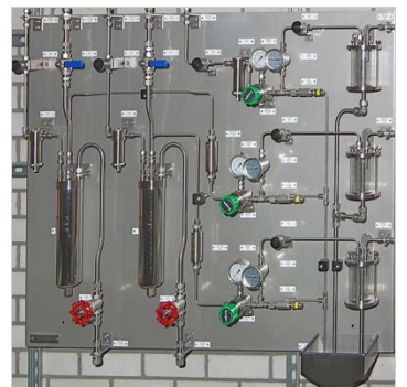
3-stream sample conditioning
