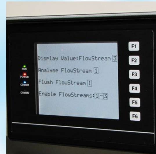
The display shows the stream being analysed and also the stream that are enabled.
