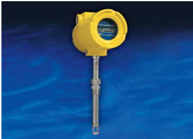
Model ST98 is an insertion flow meter for pipe sizes from 2 1/2 to 42 inches [64 to 1066 mm]. Typical calibration range is from 0.75 to 600 SFPS [0.21 to 172 NMPS]. 1
