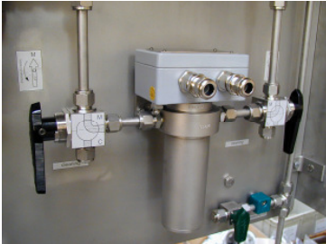
DIMF 1.3 (left) on a pedestal mounted density skid (right)
